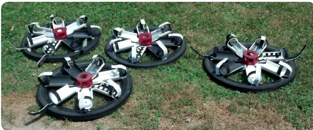
The wheels may be removed and directly exposed to sunlight to maximize solar UV radiation disinfection.
